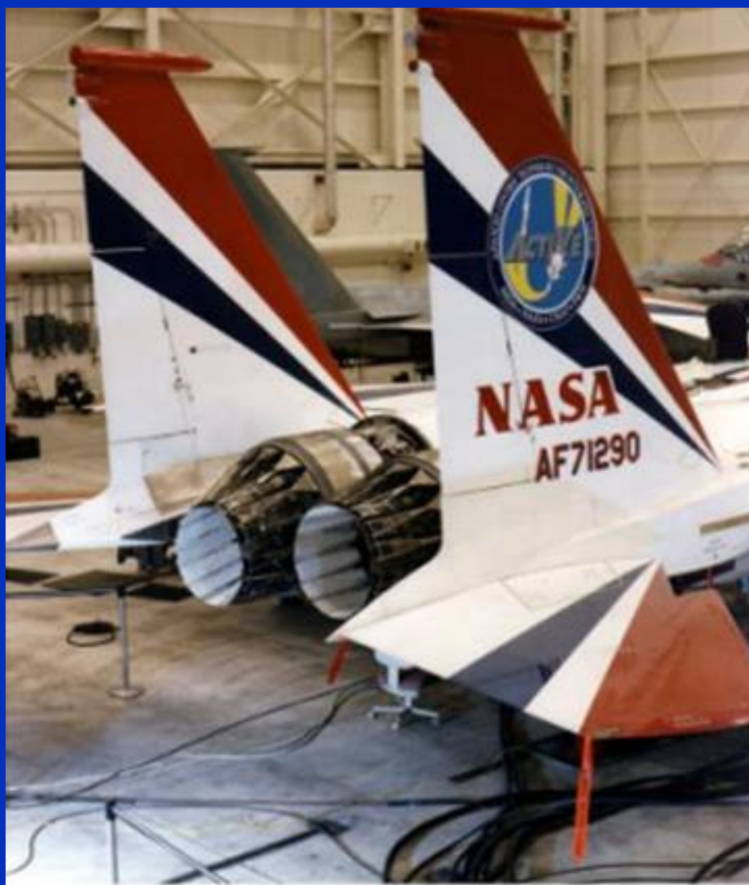
Dryden Flight Research Center EC95-43273-4 Photographed 1995 F-15 Advanced Control Technology for Intergrated Vehicles (ACTIVE) showing thrust-vectoring nozzles. NASA photo
