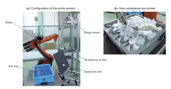
Fig. 1 Bin picking robotics using 3D object recognition
