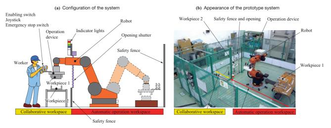
Fig. 3 Concept of hand guiding system
