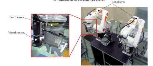
Fig. 4 Cell production robot system
