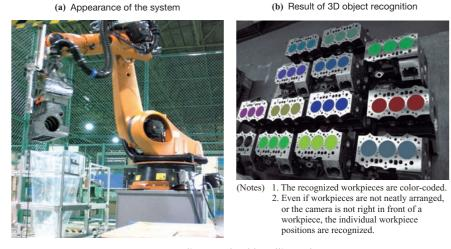
Fig. 2 Medium payload handling robot
