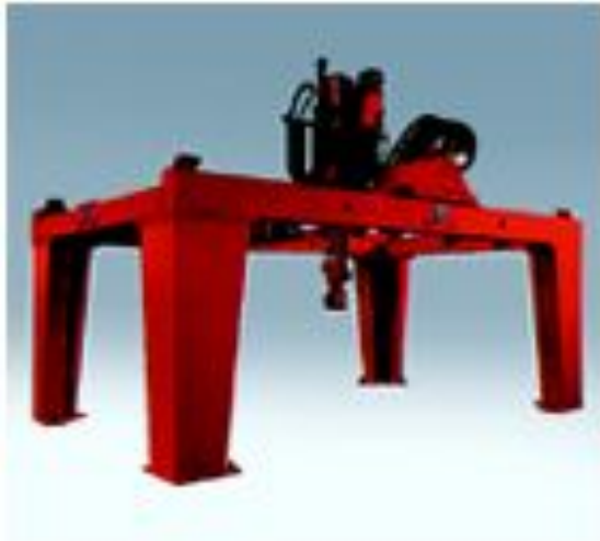
Comau Mast gantry robot (payload up to 560 kg)
