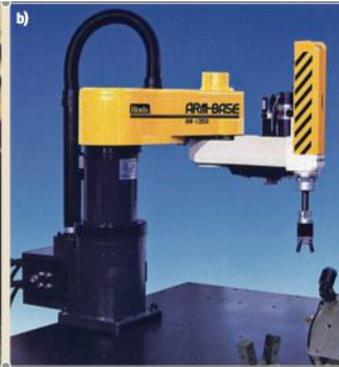
Hirata AR-300 (1978) first SCARA robot
